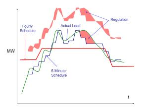
Figure 4: Regulation Requirement (Red Shaded Area).
