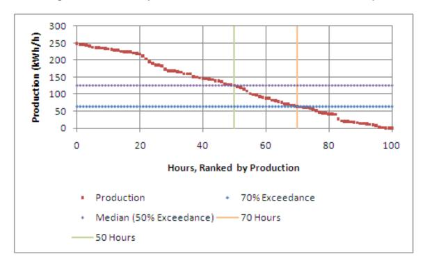
Figure 8: Conceptual Illustration of the Exceedance Concept<sup>45</sup>
