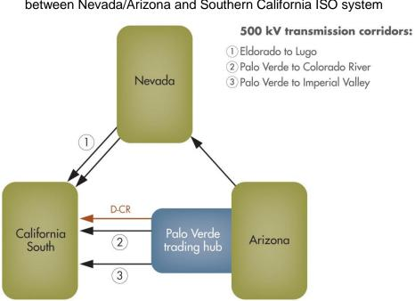
Figure 5.7-12: 500 kV transmission connections between Nevada/Arizona and Southern California ISO system
