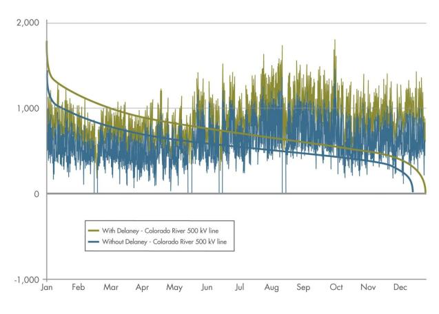
Palo Verde - Colorado River 500 kV — simulated MW flow in 2023
