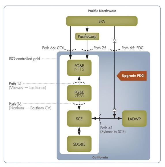
The present PDCI path rating is 3,100 MW. Currently, BPA's PDCI Upgrade Project is in progress. This will increase the PDCI rating by 120 MW to 3,220 MW. This planning study analyzes a future potential network upgrade with an additional 500 MW increase to the PDCI rating.
