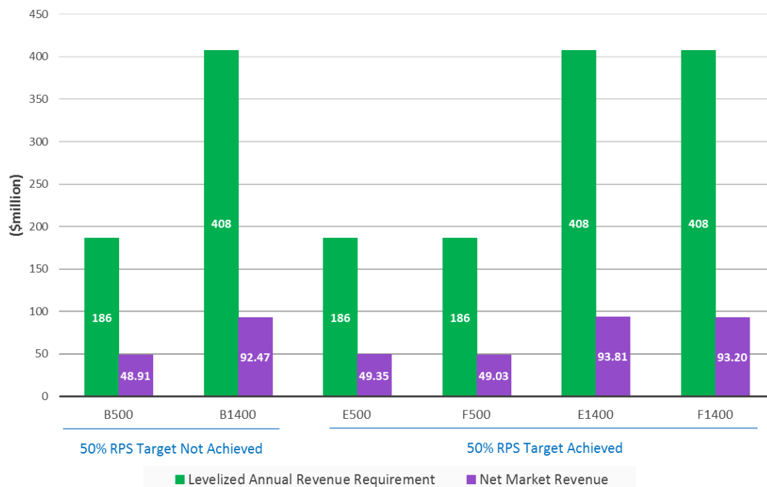
Figure 6.5-7: Levelized Annual Revenue Requirement and Net Market Revenue of the New Pumped Storage Resource in 2026
