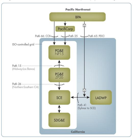
Figure 5.7-20: Pacific Northwest – California (NWC) system configuration
