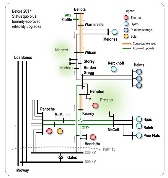
Figure 5.7-12: Greater Fresno Area (GFA) 230 kV system – status quo before 2017
