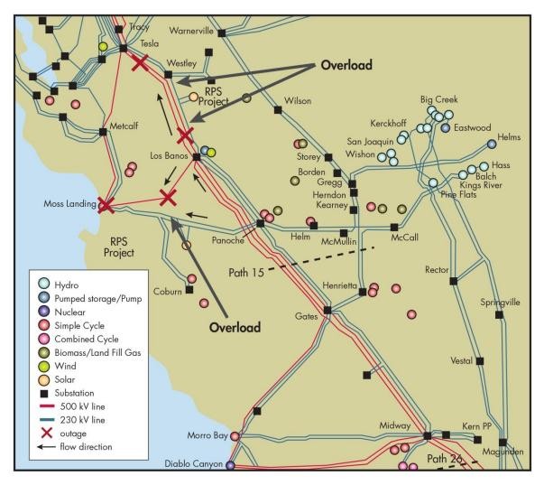
Figure 4.2:12: Overloads in Central PG&E area
