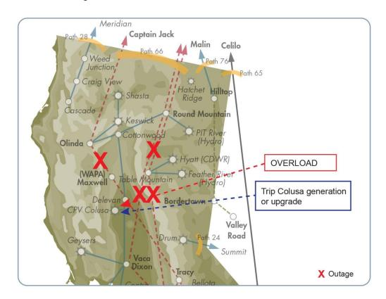
Figure 4.2:11: Delevan-Cortina 230 kV line overload
