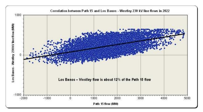
Figure 5.7-10: Correlation between Path 15 and Los Banos – Westley 230 kV line flow
