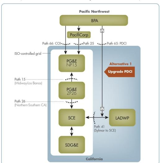
Figure 5.7-21: Proposed network upgrade under this study (Alternative 1: Increase PDCI rating from 3220 to 3280 MW)
