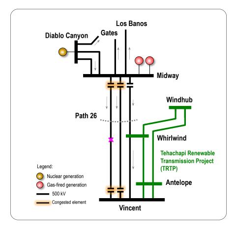
Figure 5.7-2: One-line diagram of the Path 26 area
