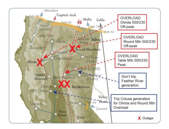
Figure 3.5-1: Northern California 500/230 kV transformer overloads
