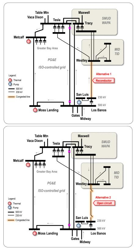
Figure 5.7-7: Alternatives of proposed network upgrades under the LBN study
