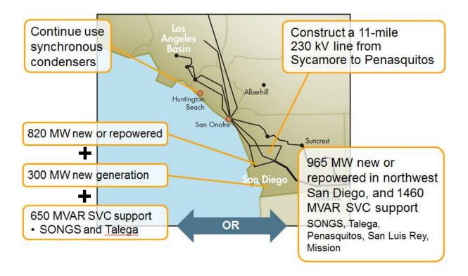
Figure 3.5-3: Mid-term mitigation alternatives for loss of SONGS
