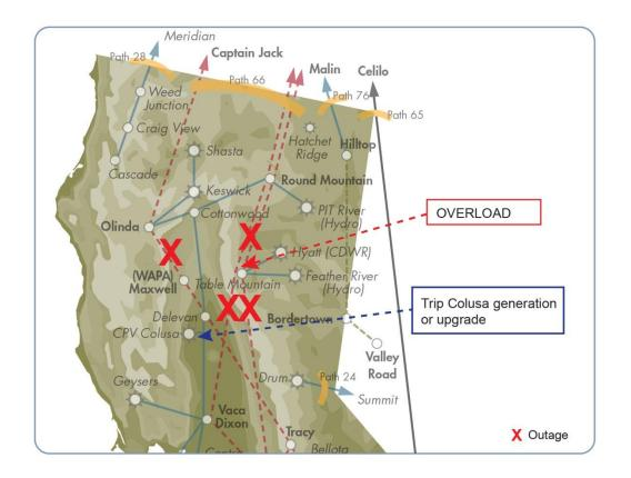
Figure 3.5-2: Delevan-Cortina 230 kV line overload
