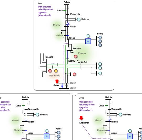
Figure 5.7-14: Alternatives of potential network upgrades analyzed in this study
