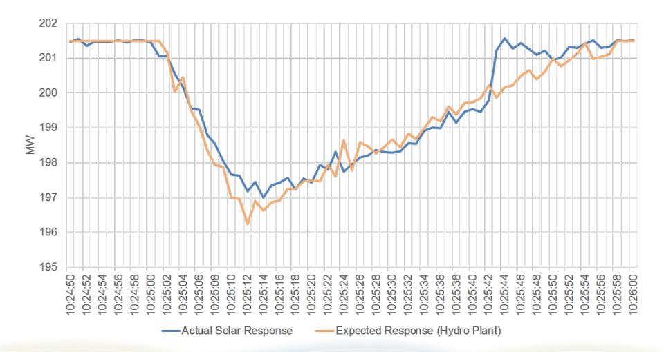
Ability of solar plant to respond and arrest frequency decline similar to a hydro plant for a **low** frequency event
