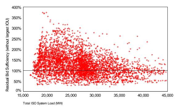
Figure 7-13. RSI for Pivotal IOU in Spinning Reserves v. Total ISO Load
