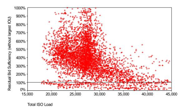
Figure 7-17. RSI for Pivotal IOU in Replacement Reserves v. Total ISO Load
