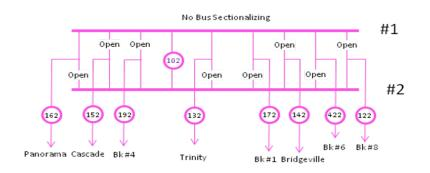
Cottonwood 115kV Bus Sectionalize & Re-Arrange the Bus #1 & #2 connections (includes Bus Selector Switches Changes)
