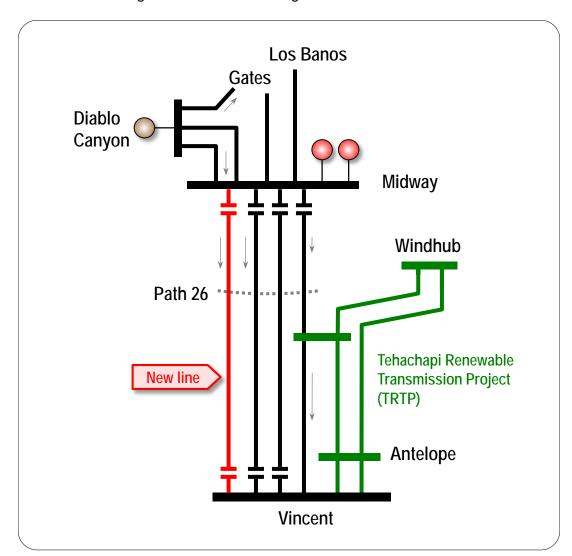
Figure 5.7-1: One-line diagram of the Path 26 area
