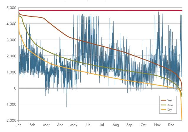
Figure 5.7-7: Simulated power flow on Path 65 (PDCI) (navy blue = hourly chronological flows; others = duration exceedance curve)
