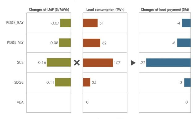
Figure 5.7-11: LMP and load payment changes with addition of the Harry Allen – Eldorado 500 kV line
