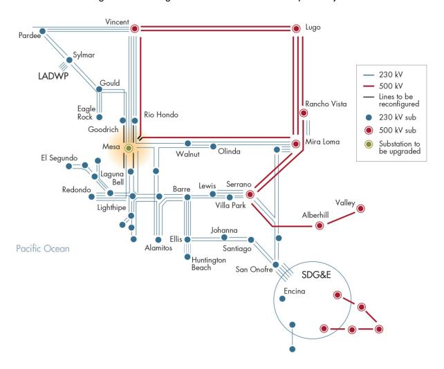
Figure 2.6.3: Diagram of the Mesa 500 kV Loop-in Project
