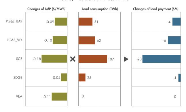
Figure 5.7-16: LMP and load payment changes with addition of the Delaney – Colorado River 500 kV line
