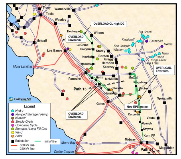
Figure 4.2–3. Off-peak Overloads in the Fresno Area under Normal Conditions
