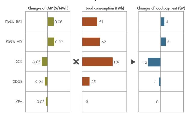
Figure 5.7-4: LMP and load payment changes with addition of the Midway – Vincent 500 kV line #4
