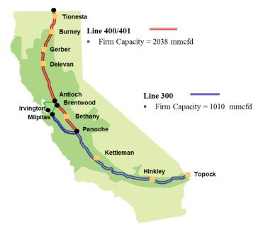
Figure 6.3-5: Northern California backbone gas pipeline and capacity
