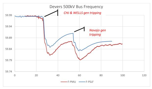
Figure 6.2-6: Comparison of Bus Frequency
