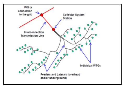
Figure 6.2-3: Configuration of a Wind Farm (or solar PV plant)
