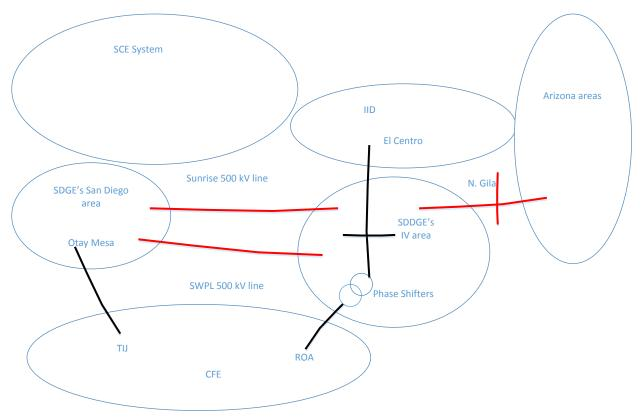
Figure 4.7-2: SDGE/IID/CFE area electrical interconnections
