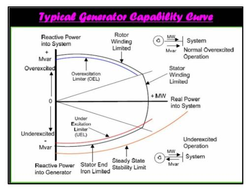
Figure 6.2-2: Reactive Capability Curve of a Synchronous Generator
