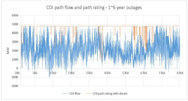
Figure 4.7-1: COI path flow and path rating with 1~6 year outages modeled
