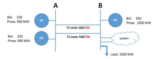
Currently, the market enforces a 750 MW emergency limit on transmission line T1 for the loss of transmission line T2. The total normal transfer limit from A to B is 1000 MW (500 MW on T1 plus 500 MW on T2). The total emergency transfer limit from A to B is 1500 MW (750 MW on T1 plus 750 MW on T2); however, given the loss of T2, an emergency transfer limit from A to B of 750 MW is enforced today.
