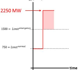
Given the loss of the generator G1 at A, path AB would be loaded above its emergency rating of 1500 MW. A secure dispatch would ensure that path AB does not load above its emergency rating given a single contingency event. The dispatch that achieves this goal is shown below.
