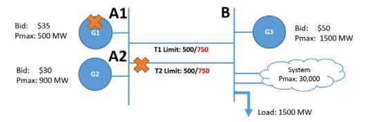
As shown using orange X's above, a remedial action scheme is defined such that if transmission line T2 is lost, generator G1 will be tripped offline. The total normal transfer limit from A to B is 1,000 MW (500 MW on T1 plus 500 MW on T2). The total emergency transfer limit from A to B is 1,500 MW (750 MW on T1 plus 750 MW on T2); however, given the simultaneous preventive loss of T2 and G1, an emergency transfer limit between A and B of 750 MW will be enforced.
