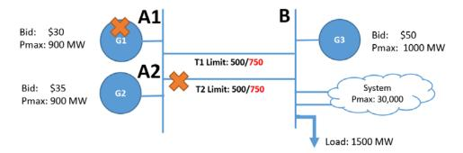
As shown using orange X's above, a remedial action scheme is defined such that if T2 is lost, G1 will be tripped offline. The total normal transfer limit between A and B is 1000 MW (500 MW on T1 plus 500 MW on T2). The total emergency transfer limit between A and B is 1500 MW (750 MW on T1 plus 750 MW on T2); however, given the simultaneous preventive loss of T2 and G1, an emergency transfer limit between A and B of 750 MW will be enforced.
