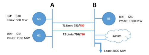
The total normal transfer limit between A and B is 1,500 MW (750 MW on T1 plus 750 MW on T2). The total emergency transfer limit between A and B is 1,500 MW (750 MW on T1 plus 750 MW on T2); however, given the loss of T2, an emergency transfer limit between A and B of 750 MW will be enforced. In this example, the transmission system is designed such that there is no additional transfer capability on T1 or T2 above normal limits.
