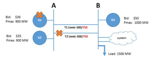
As shown using orange X's above, a remedial action scheme is defined such that if T2 is lost, G1 will be tripped offline. The total normal transfer limit between A and B is 1000 MW (500 MW on T1 plus 500 MW on T2). The total emergency transfer limit between A and B is 1500 MW (750 MW on T1 plus 750 MW on T2); however, given the preventive loss of T2+G1, an emergency transfer limit between A and B of 750 MW will be enforced.
