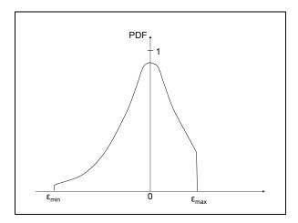
Figure 1: Unbiased Truncated Normal Distribution
