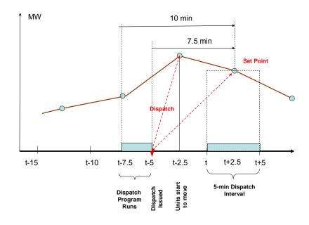
Figure 3: CAISO Real Time Dispatch Timeline
