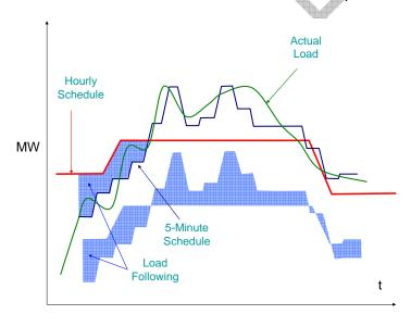
Figure 17: Load Following Requirement shown as blue shaded area
