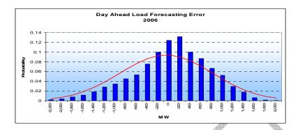
Figure 2: CAISO DA Load Forecasting Error
