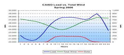
Figure 4: Actual System Load, Wind Generation and Solar Generation for Spring 2006)
