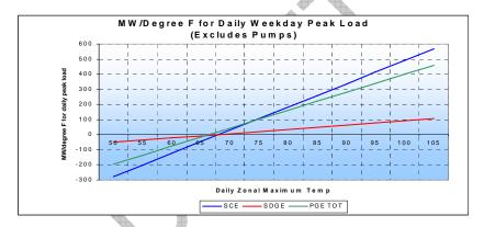
Figure 1: Temperature vs. Peak Load Variation
