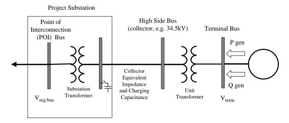
Figure 1: Wind Plant Equivalent Model.
