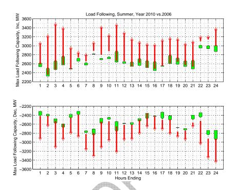
Figure 18: Load Following Capacity Requirement
