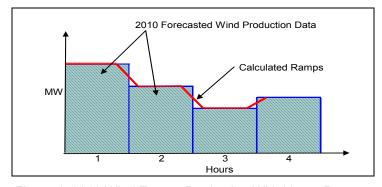
Figure 1: 2010 Wind Energy Production With Linear Ramps
