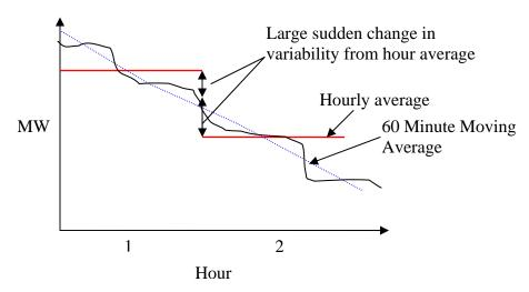
Figure 2: Sample Wind production with hourly average, and moving average
