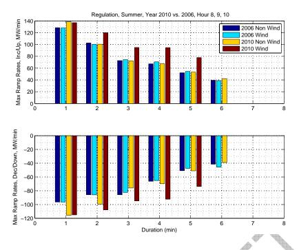
Figure 24: Regulation Ramp Duration
