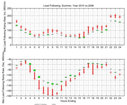
Figure 19: Load Following Ramping Requirement
