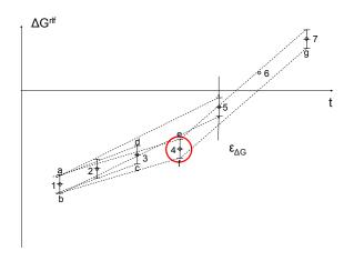
Figure 8: "Swinging Door" Algorithm - Idea
