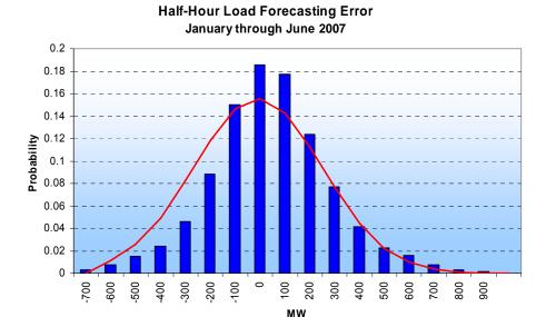
Figure 3: Comparison of Half-Hour Load Forecast Error with Theoretical Distribution
