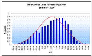
Figure 13: Summer load error distributions vs. Theoretical load error distributions
