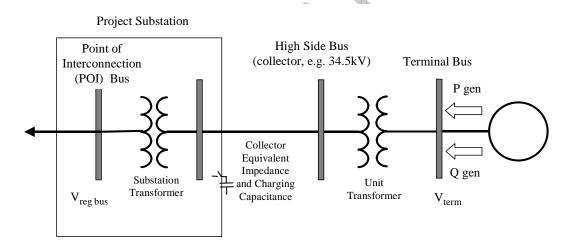
Figure 1: Wind Plant Equivalent Model
