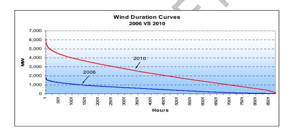
Figure 1: Actual Wind Generation for 2006 vs. Expected Wind Generation for 2010
