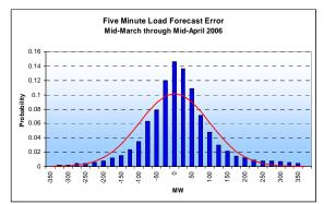
Figure 15: Comparison of five-minute load forecast error and theoretical error distribution
