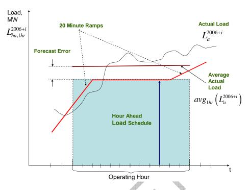
Figure 14: CAISO Simulated Hour-Ahead Load Schedule (Red Line) with Ramps
