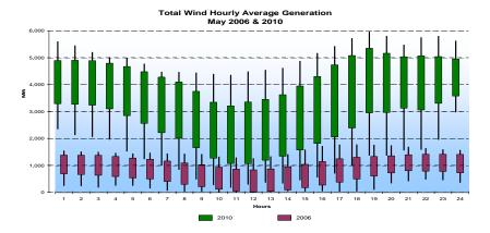
Figure 3: Actual 2006 Hourly Wind Generation vs. Expected 2010 Hourly Wind Generation
