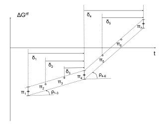
Figure 9: "Swinging Window" Algorithm - Obtaining Regulation, Ramps, and Their Duration
