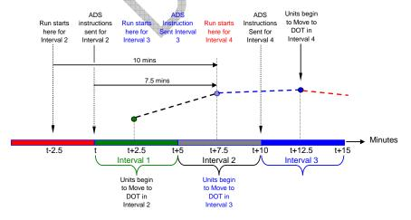
Figure 16: MRTU Timeline for five-Minute Dispatch
