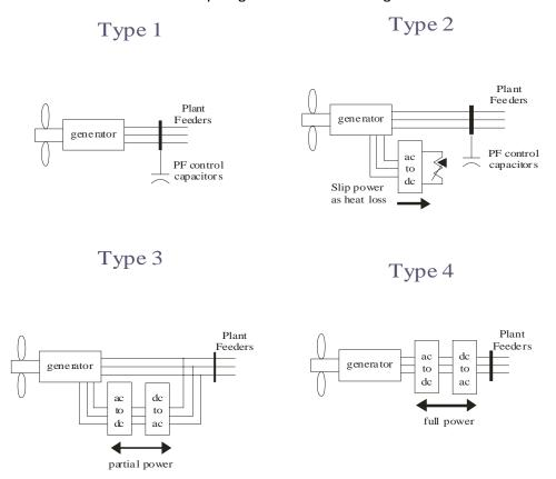
Figure 2: WECC Standard Wind Turbine Model Types.
