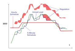
Figure 21: Regulation Requirement shown as the red shaded area
