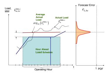
Figure 5: Probability Density Function (PDF) of the Load Forecast Function (Red Line)
