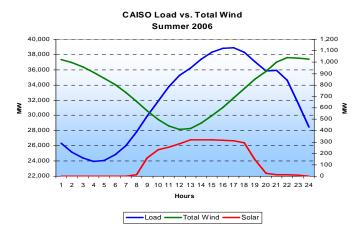
Figure 7: Actual System Load, Wind Generation & Solar Generation for Summer 2006
