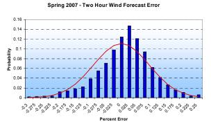
Figure 1b: Spring Forecasting Error
