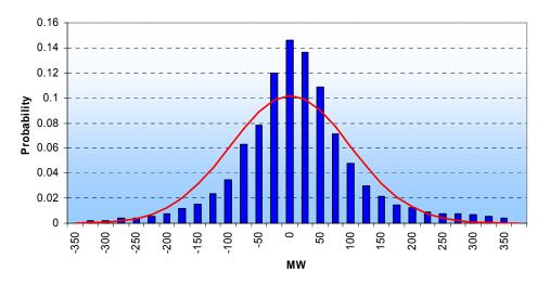
Figure 4: Comparison of five-minute Load Forecast Error and Theoretical Error Distribution
