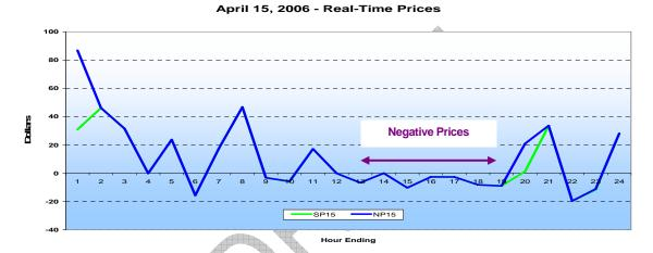
Figure 27: Real Time Prices During Overgeneration Conditions
