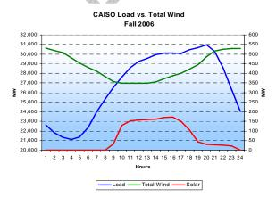
Figure 9: Actual System Load, Wind Generation and Solar Generation for Fall 2006
