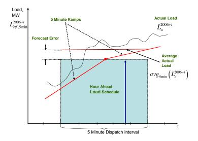
Figure 6: CAISO Simulated Real Time Load Forecast (Red Line)
