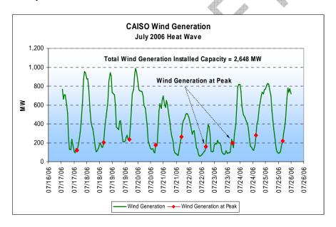
Figure 2: CAISO Wind Generation during the 2006 Heat Wave
