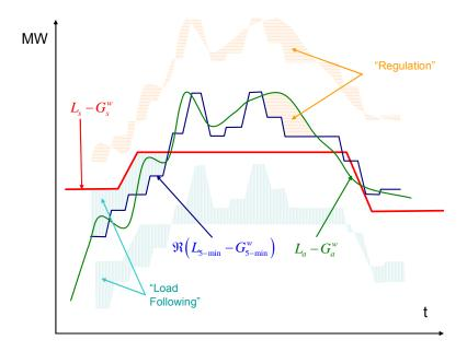
Figure 7: Separation of Regulation from Load Following Based on Simulated Hour Ahead Schedule
