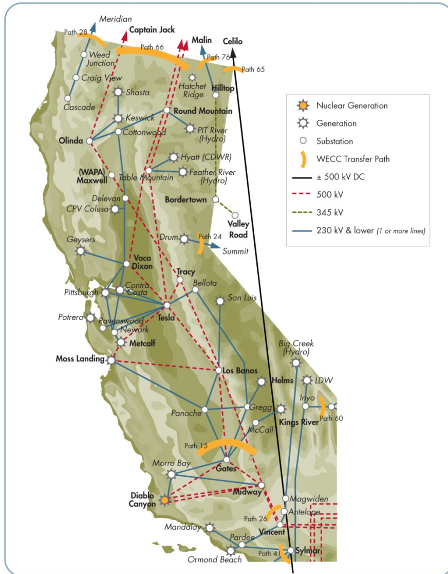
Figure 2.4-1: Map of PG&E bulk transmission system
