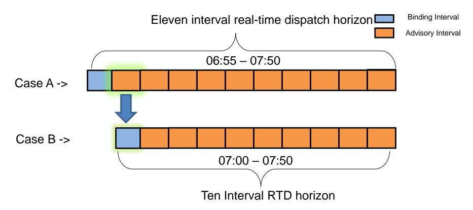
Compare results for 7:00 to 7:05 real-time dispatch interval between case A and case B
