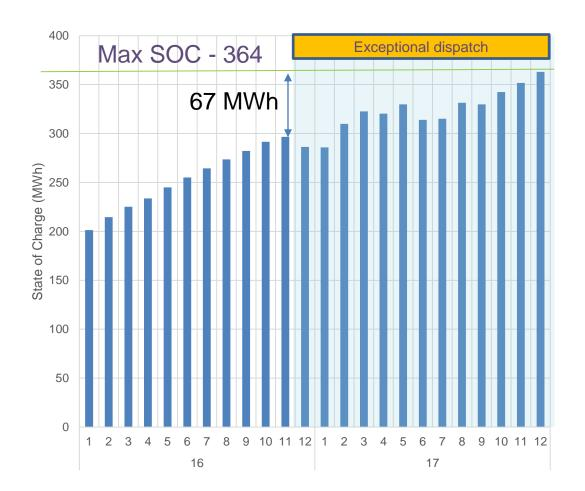
At hour ending 16 interval 11, the initial state of charge was 297 MWh.
