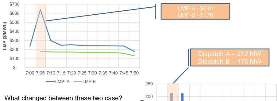
Active flow management on Lugo – Victorville 500 kV line resulted in lower level of congestion and drove lower marginal congestion price, resulting in a lower real-time dispatch
