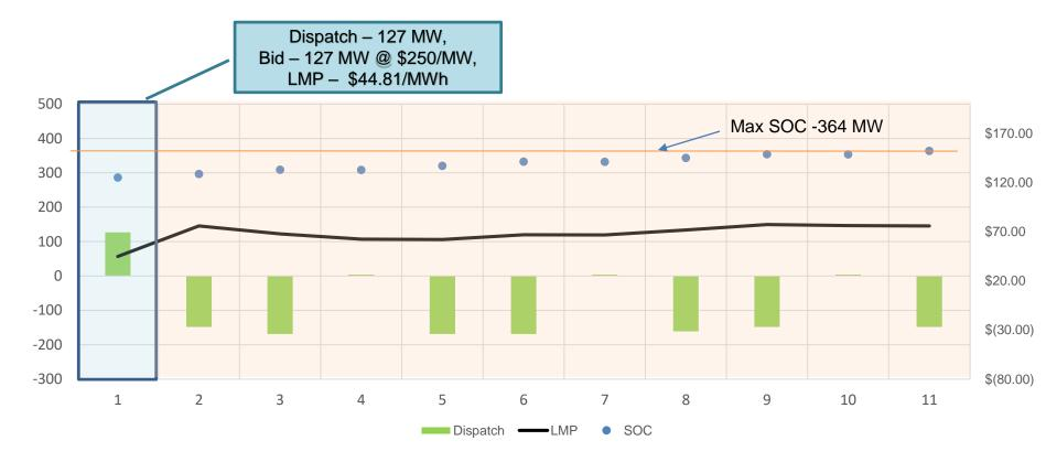
Binding Interval LMP is \$44.81/MWh whereas its discharge offer is \$250. The resource is discharged uneconomically due to a fixed ED to charge the resource at 184 MW instead of 79 MW and a software issue
