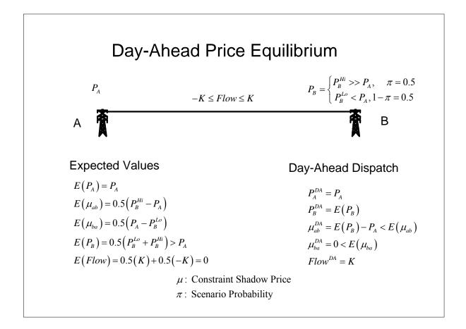
The transmission system is the same day ahead and in real time. The conditions at node A imply a net supply-and-demand condition that yields a constant price,  $P_A$  under all real-time conditions.
