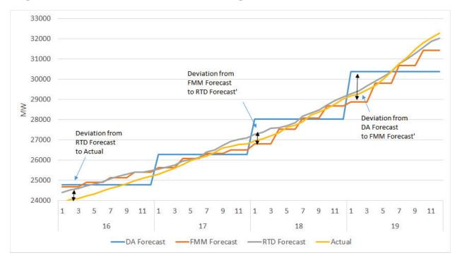
Figure 2: Forecast error and load following needs between IFM and actual needs
