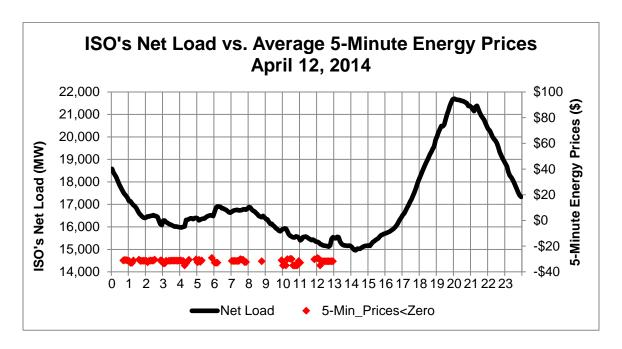
Figure 1 - Actual Net Load Curve for April 12, 2014
