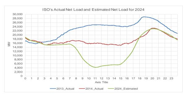
Figure 2: Net Load Curves (2013, 2014 and 2024 Estimated)
