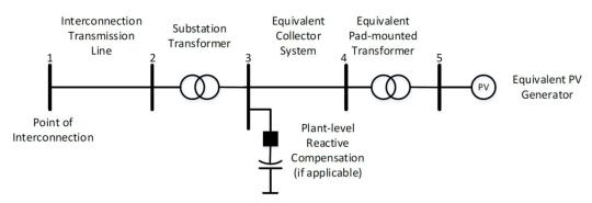
Figure 1: Single-Generator Equivalent Power Flow Representation for a Solar PV Power Plant
