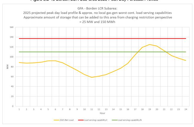
Figure 3.2-48 Borden LCR Sub-area 2025 Peak Day Forecast Profiles
