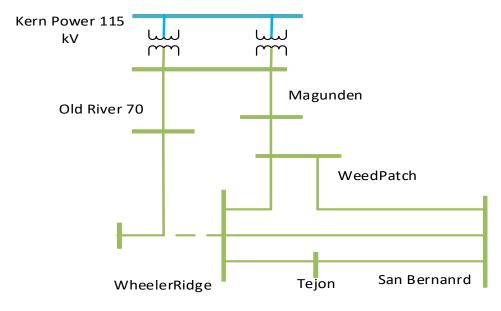
Figure 3.2-63 Kern 70 kV LCR Sub-area
