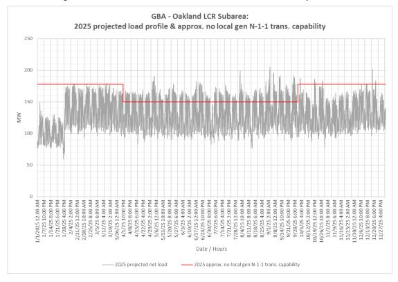
Figure 3.2-35 Oakland LCR Sub-area 2025 Forecast Hourly Profiles
