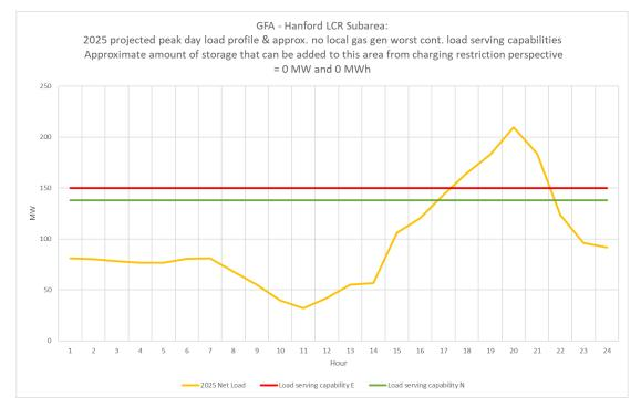
Figure 3.2-43 Hanford LCR Sub-area 2025 Forecast Hourly Profiles
