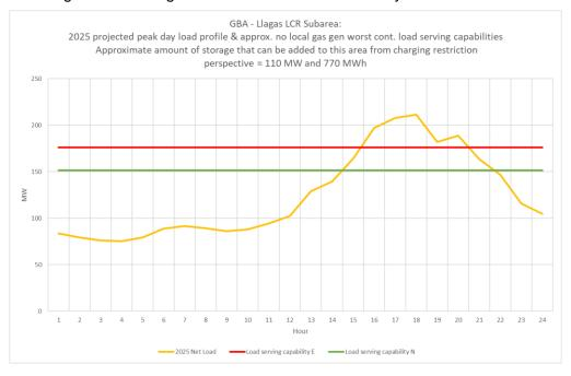
Figure 3.2-27 Llagas LCR Sub-area 2025 Peak Day Forecast Profiles
