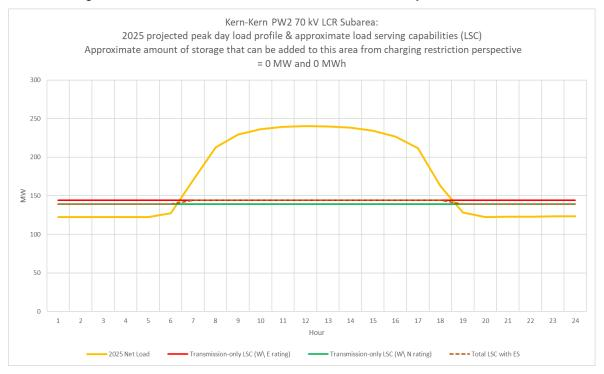
Figure 3.2-65 Kern 70 kV LCR Sub-area 2025 Forecast Hourly Profiles
