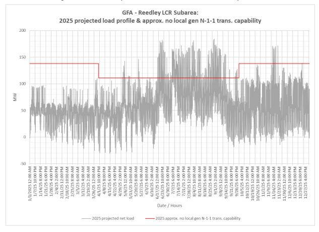
Figure 3.2-52 Reedley LCR Sub-area 2025 Forecast Hourly Profiles
