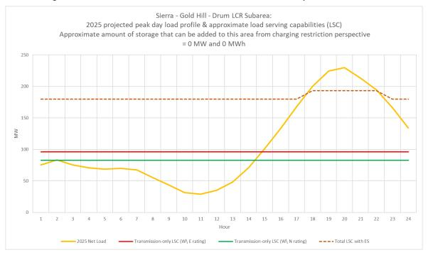
Figure 3.2-19 Gold Hill-Drum LCR Sub-area 2025 Forecast Hourly Profiles
