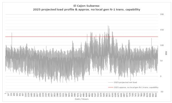
Figure 3.2-94 El Cajon LCR Sub-area 2025 Annual Load Forecast Profiles
