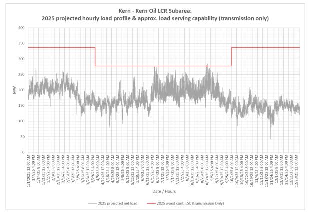
Figure 3.2-70 Kern Oil LCR Sub-area 2025 Forecast Hourly Profiles
