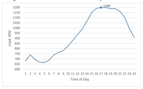
Figure 3.2-76 Vestal LCR Sub-area 2025 Peak Day Forecast Profiles
