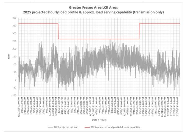
Figure 3.2-55 Panoche LCR Sub-area 2025 Forecast Hourly Profiles
