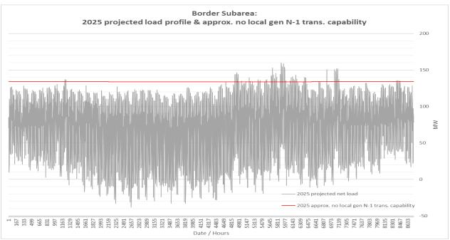
Figure 3.2-97 Border LCR Sub-area 2025 Annual Load Forecast Profiles
