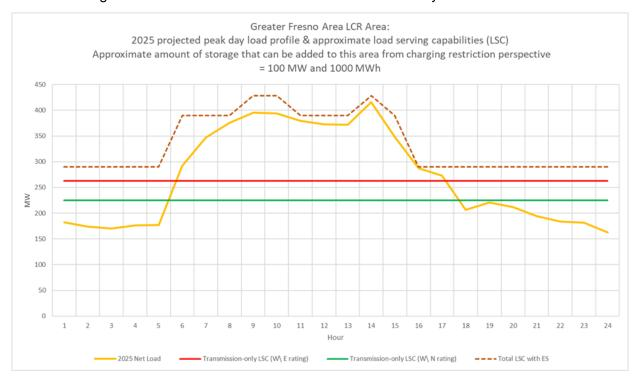
Figure 3.2-54 Panoche LCR Sub-area 2025 Peak Day Forecast Profiles
