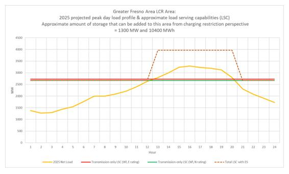
Figure 3.2-61 Fresno LCR Area 2025 Forecast Hourly Profiles
