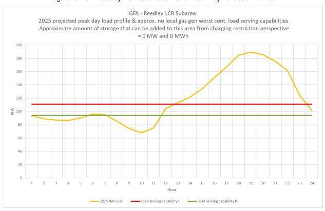
Figure 3.2-51 Reedley LCR Sub-area 2025 Peak Day Forecast Profiles
