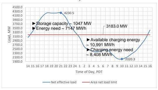
Figure 3.2-82 Big Creek/Ventura Local Capacity Energy Storage Analysis with Sylmar–Pardee Project
