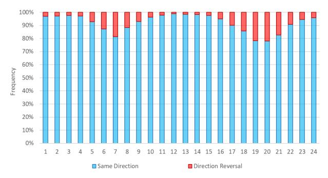
Figure 66: Frequency of direction reversal of net load error due to operator adjustments
