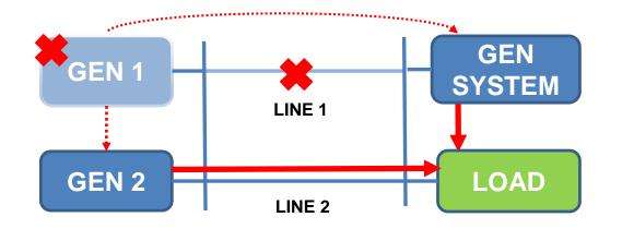
GEN 1 is part of remedial action scheme and trips off if LINE 1 or LINE 2 go out
