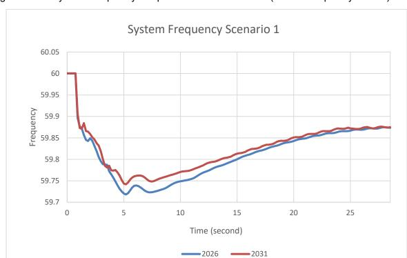
Figure 6.3-3: System Frequency Response for Baseline Case (No IBR frequency control)
