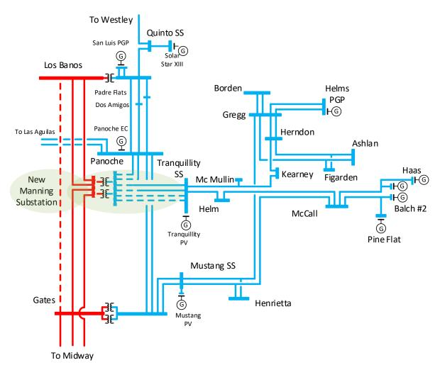
Figure 3.5-2: Manning 500/230 kV substation interconnection
