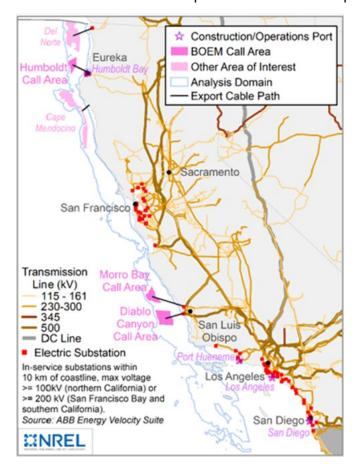
Figure 3.7-1: Offshore Wind Development Location Assumptions 134
