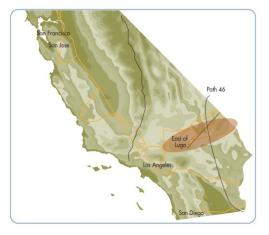
Nevada and Arizona; is a part of Path 46 (West of River), and is heavily integrated with LADWP and other neighboring transmission systems. The Harry Allen-Eldorado 500 kV line went in-service in July 2020 and is now part of the EOL system.
