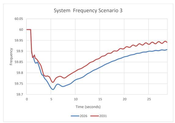
Figure 6.3-5: System Frequency Response under Sensitivity Case (~10% headroom)
