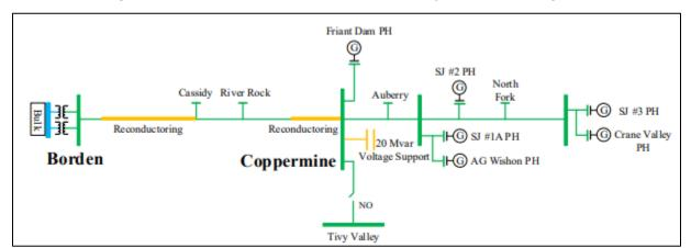
Figure - Coppermine 70 kV Reinforcement Project one-line diagram.
