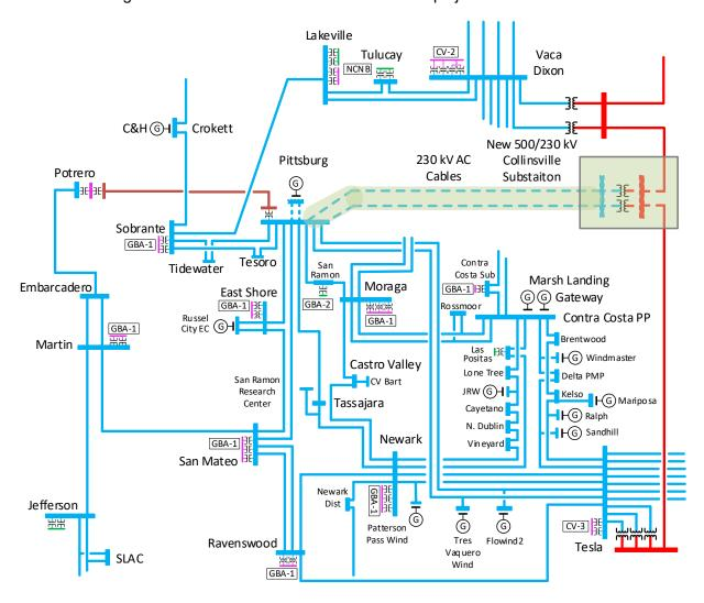
Figure 3.5-1: Collinsville 500/230 kV substation project interconnection
