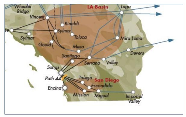
Figure 2.6-1: Southern California Bulk Transmission System
