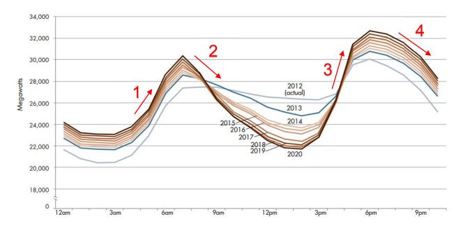
Figure 2: net load curve showing ramping needs – January 11
