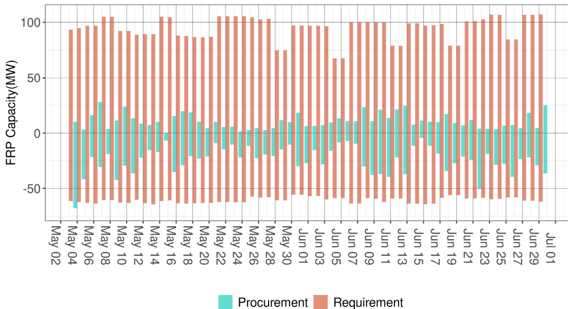
Figure 7: Daily average requirement and procurement of upward and downward flexible ramping in FMM
