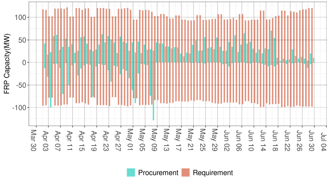
Figure 7: Daily Average flexible ramping Up and Down requirement and procurement in the FMM for the LADWP BAA.
