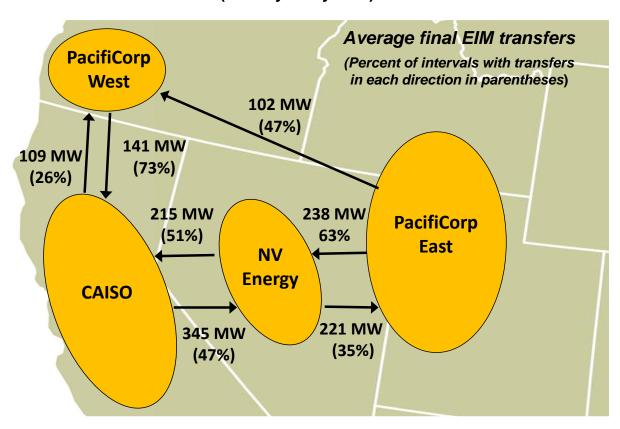
Figure 5. Final net EIM transfers between balancing areas (January – May 2016)
