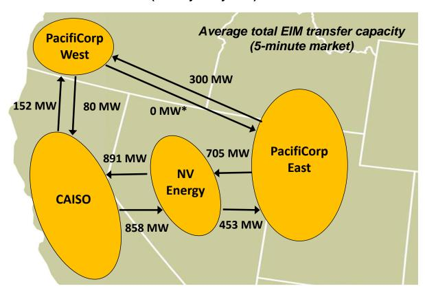
Figure 4. Total average transfer capacity between EIM balancing areas (January – May 2016)
