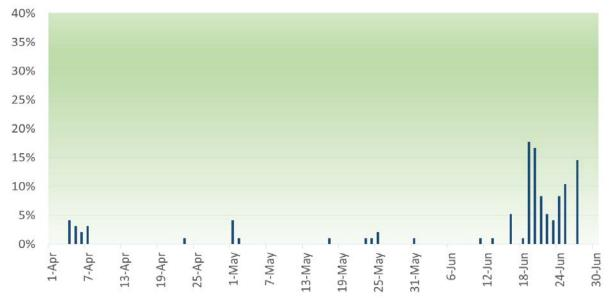
Figure 47: Frequency of Flexible Ramping Sufficiency Test Failures in the PAC West BAA
