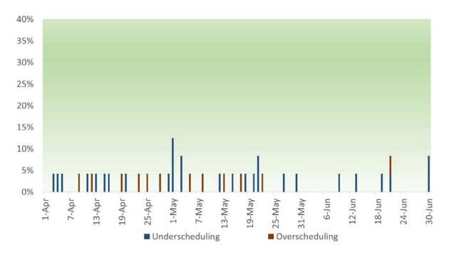
The APS BAA passed the balancing test in 94 percent of the hours and approximately half of the failures were for under-scheduling conditions. For the PSE BAA, the passing rate was approximately 97.5 percent of the hours and approximately three quarters of infeasibilities were for under-scheduling conditions.
