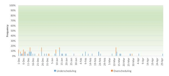
Figure 6: Frequency of Balancing test failures for NV Energy area.
