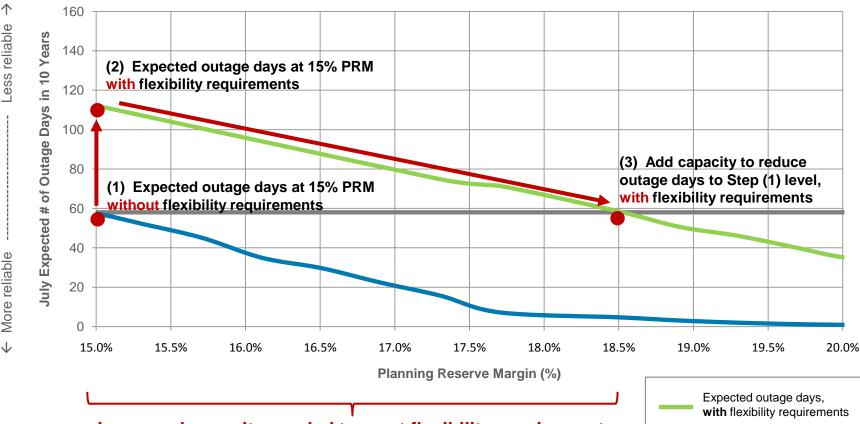
Trajectory Case: Comparison with and without flexibility requirements
