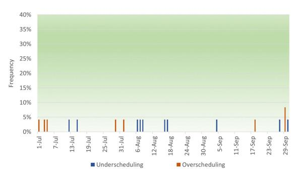
The APS BAA passed the balancing test in 98.1 percent of the hours and approximately 57 percent of the failures were for under-scheduling conditions. For the PSE BAA, the passing rate was 98.5 percent of the hours and 68.8 percent of infeasibilities were for under-scheduling conditions.
