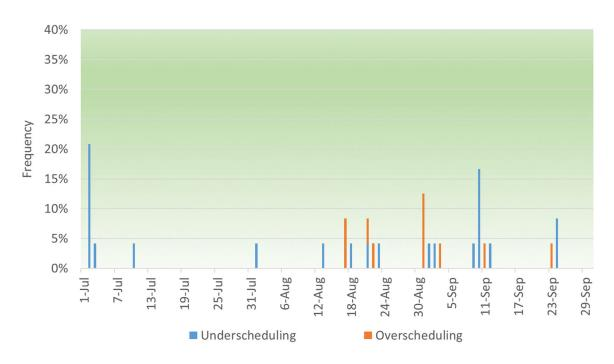
The IPCO BAA passed the balancing test in 99.7 percent of the hours and approximately 71.4 percent of the failures were for under-scheduling conditions. For the PGE BAA, the passing rate was 99.2 percent of the hours and approximately 53 percent of infeasibilities were due to under-scheduling conditions.
