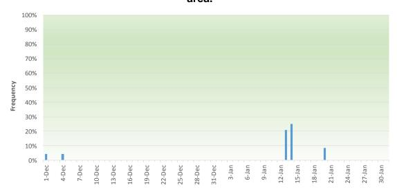
Figure 7: Frequency of flexible ramp sufficiency test failures in NV Energy area.
