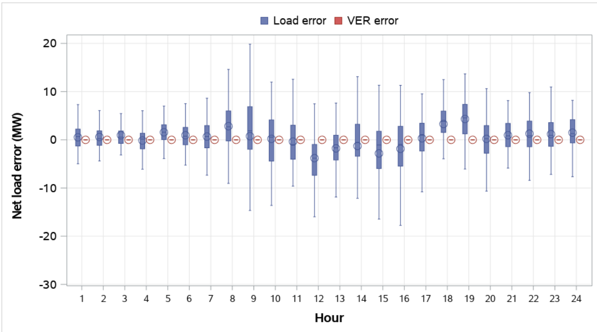
Figure 8.55 Turlock Irrigation District distribution of RSE and RTD load and VER error (weekdays, March 2022)
