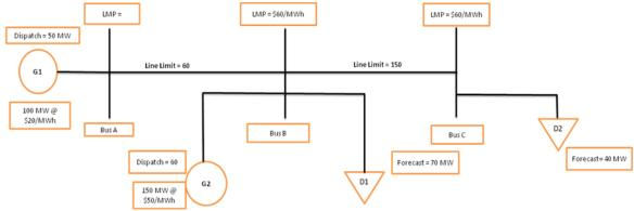
As seen from Table 15, the generator G1 has a net decrement of 10 MW, that is, its output in the real-time is reduced from 60 MW to 50 MW. A net decrement for a generator results in a positive quantity which is equivalent to a demand.
