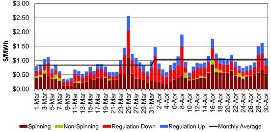
Figure 74 below shows the total system (IFM, HASP and RTUC) average cost to load for ancillary services procurement in the market. The average cost to load is calculated as: average ((total hourly cost of procurement for all four ancillary services) / (total hourly ISO load)).
