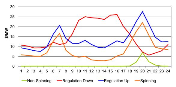
Figure 68 illustrates the real-time daily average price for ancillary services, including the average price for regulation up and regulation down procured in RTUC, and the average price for spinning and non-spinning procured in both RTUC and HASP. The average price for each type of ancillary services is calculated as: hourly average of [sum (non-self scheduled AS MW \* ancillary services marginal price \$/MW (ASMP)) / sum (non-self scheduled AS MW)] for each of the 15 minute intervals.
