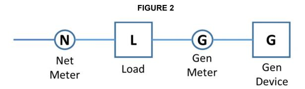
Under this configuration, the overall demand response at the location can be separated into a pure demand response (from the facility) and behind-the-meter generation energy production.
