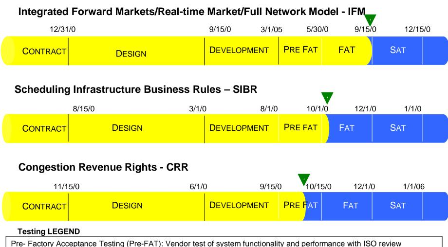
Pre- Factory Acceptance Testing (Pre-FAT): Vendor test of system functionality and performance with ISO review Factory Acceptance Testing (FAT): Formal test at vendor facility to confirm system functionality and performance with ISO Site Acceptance Testing (SAT): Formal test at ISO to confirm system functionality and performance
