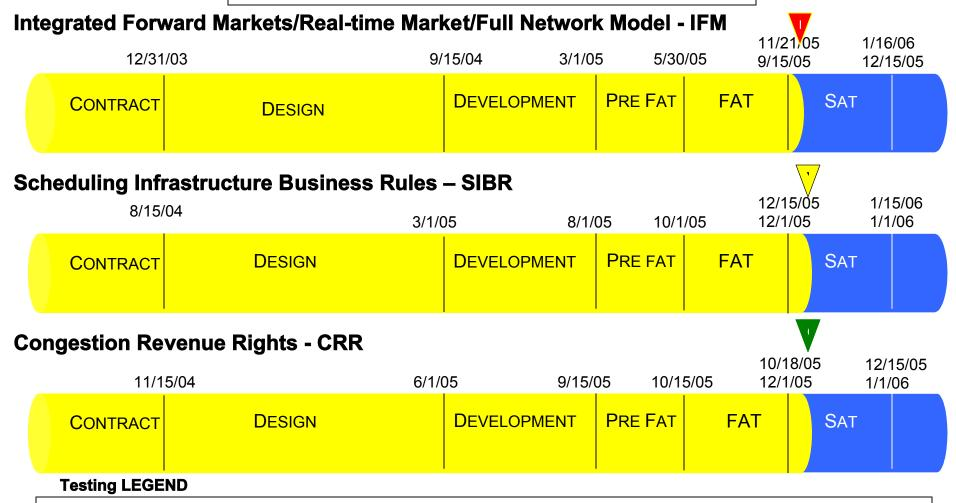
Pre- Factory Acceptance Testing (Pre-FAT): Vendor test of system functionality and performance with ISO review Factory Acceptance Testing (FAT): Formal test at vendor facility to confirm system functionality and performance with ISO Site Acceptance Testing (SAT): Formal test at ISO to confirm system functionality and performance Dates: Revised schedule dates are shown above original schedule dates.
