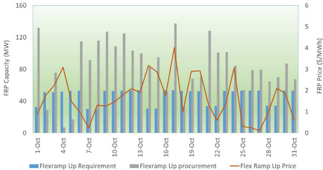
Figure 6: Daily Average requirement, procurement and price of flexible ramp up in the FMM in the PGE BAA.
