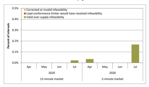
Figure 1.4 Frequency of over-supply power balance infeasibilities by month Seattle City Light
