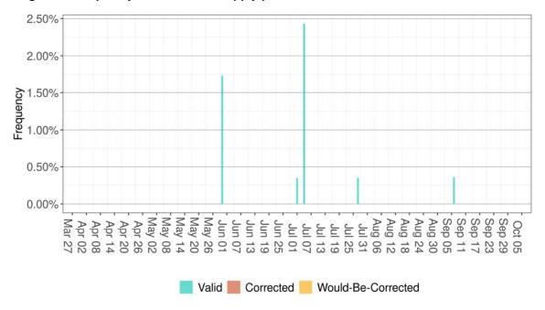
Figure 3: Frequency of RTD under-supply power balance in feasibilities in the SCL BAA.
