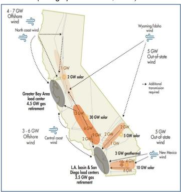
CAISO 2022-2023 Transmission Plan approved in May, 2023 met the needs of the 40 GW base case and most of the 70 GW sensitivity case needs (by 2032)
