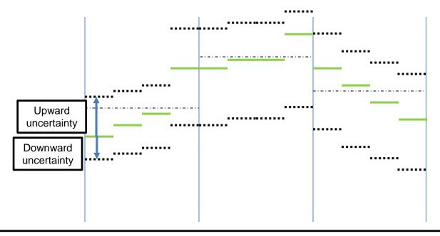
Even assuming we produce a 15-minute forecast in the day-ahead timeframe, there will be uncertainty in how much dispatchable generation is needed to meet net load.
