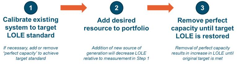
A resource's ELCC is equal to the amount of perfect capacity removed from the system in Step 3
