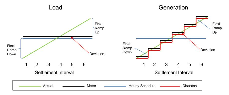
Load and Generation have equivalent measured deviations, but Load is a larger driver of flexi-ramp procurement.
