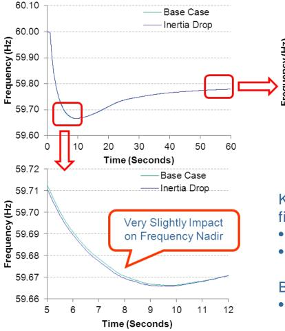
The impact of loss of inertia for 1993 MW is nearly invisible.
