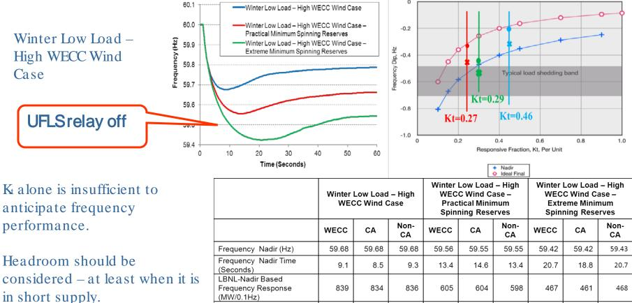
Time or time window for which settling frequency is measured becomes quite important.
