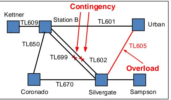
**Need:** Mitigate thermal overload on TL605 for the N-1-1 of TL602 and TL699 (SG-B ckt 1 & 2), starting in 2018, No generation available to re-dispatch
