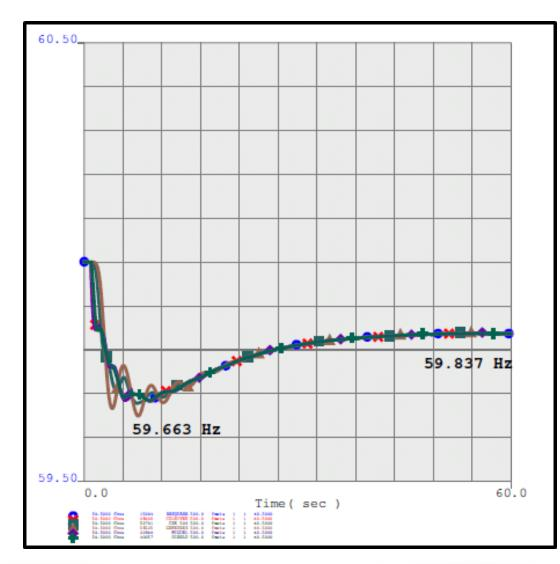
Frequency response WECC -1436 MW/0.1 Hz, within FRO
