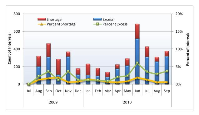
Figure 2.3 Frequency of power balance constraints in real-time intervals
