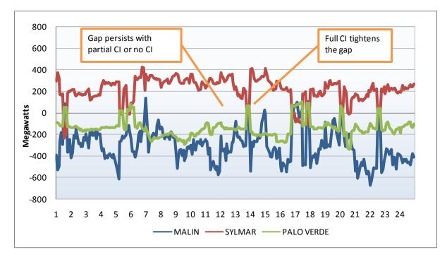
Correlating Figure 3.2 with Figure 3.1 provides a means of assessing the impact of compensating injections on the accuracy of the modeled flows over each of these inter-ties after inclusion of the compensating injections.
