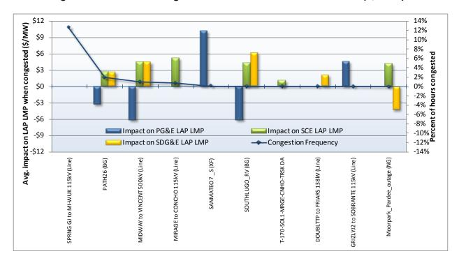
Figure 1.13 Effect of congestion on internal constraints on LAP LMPs (Q3 2010)
