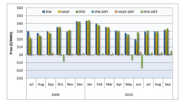
Figure 2.6 Change in monthly prices without hours when power balance constraints active (PG&E LAP, Off-peak hours)
