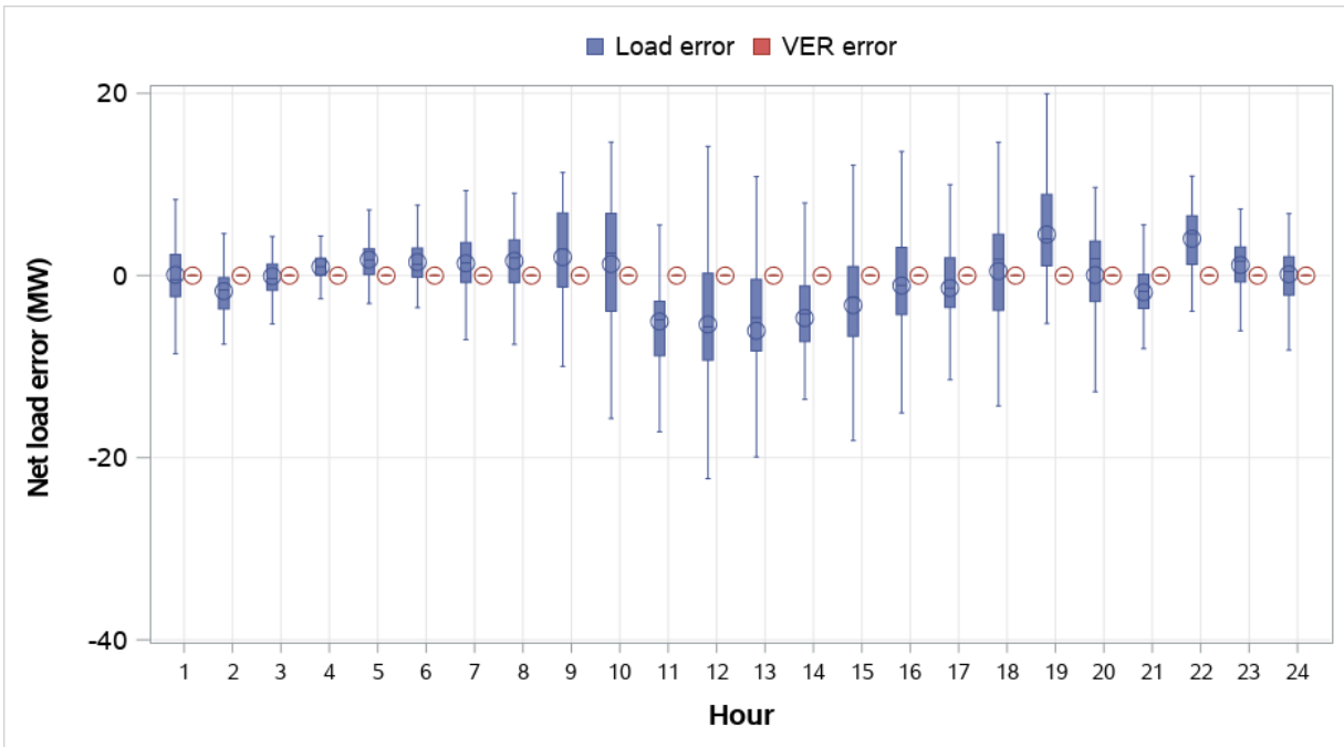
Figure 71. Turlock Irrigation District distribution of RSE and RTD load and VER error (Weekdays, October 2021)
