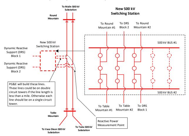
Figure 2: High level schematic diagram for Alternative 1
