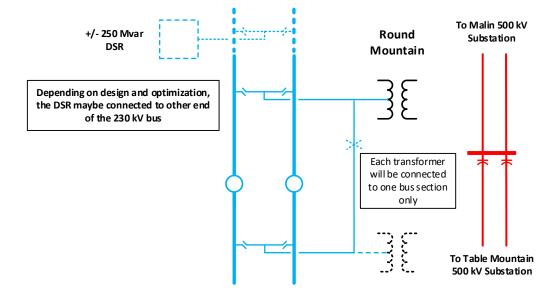
Figure 3.b: Table Mountain 230 kV Substation
