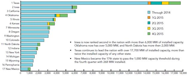
Figure 1: Installed Wind Generation Capacity, End of 2015
