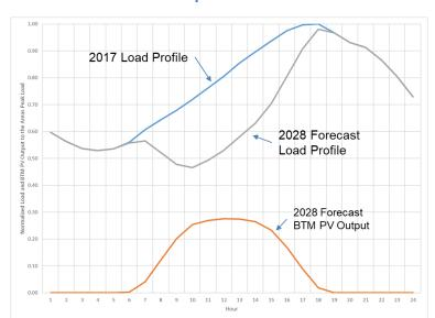
Figure 7: 2017 and 2028 (Forecasted) Load Profile with Peak normalized BTM PV Output profile
