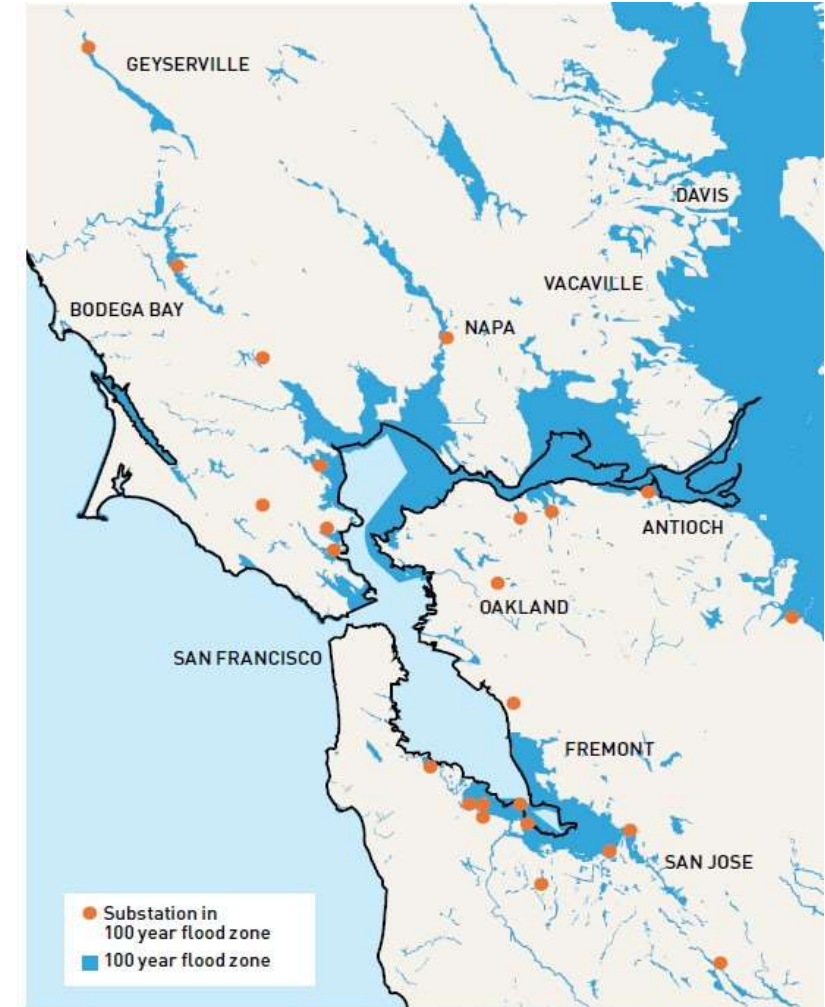
Figure 6: PG&E's electric substations identified within the 100-year FEMA flood zone
